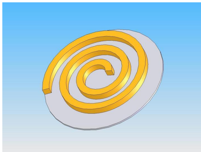
Fig 5.2: The final shape of the spiral channel silicon disk
